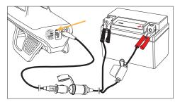
12V battery terminal charging with optional cables. Charge time: 10 hours approx.
