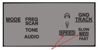
When SPEED icon is highlighted, use the Plus / Minus Menu buttons to select desired coil swing speed.
