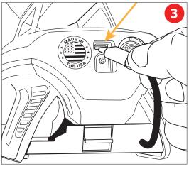
USB-C charging port is located under a weatherproof rubber flap on back of *Axiom*.
