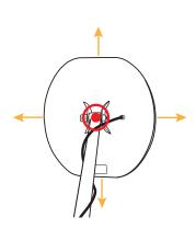
For very small, shallow targets, use either front corner of the mono coil to more precisely locate the target.
