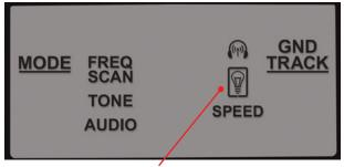
When Backlight icon is highlighted, use the Plus / Minus Menu buttons to switch on or off.
